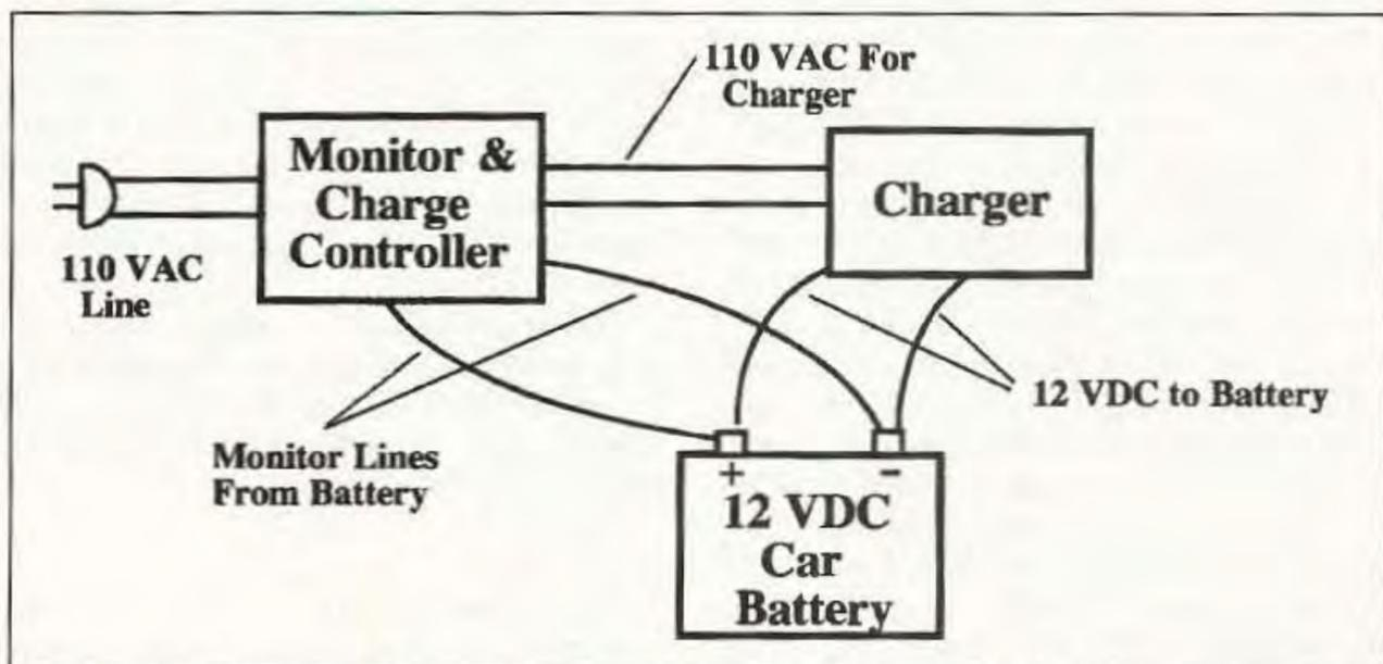
Figure 4. Connections between controller, charger and battery.
